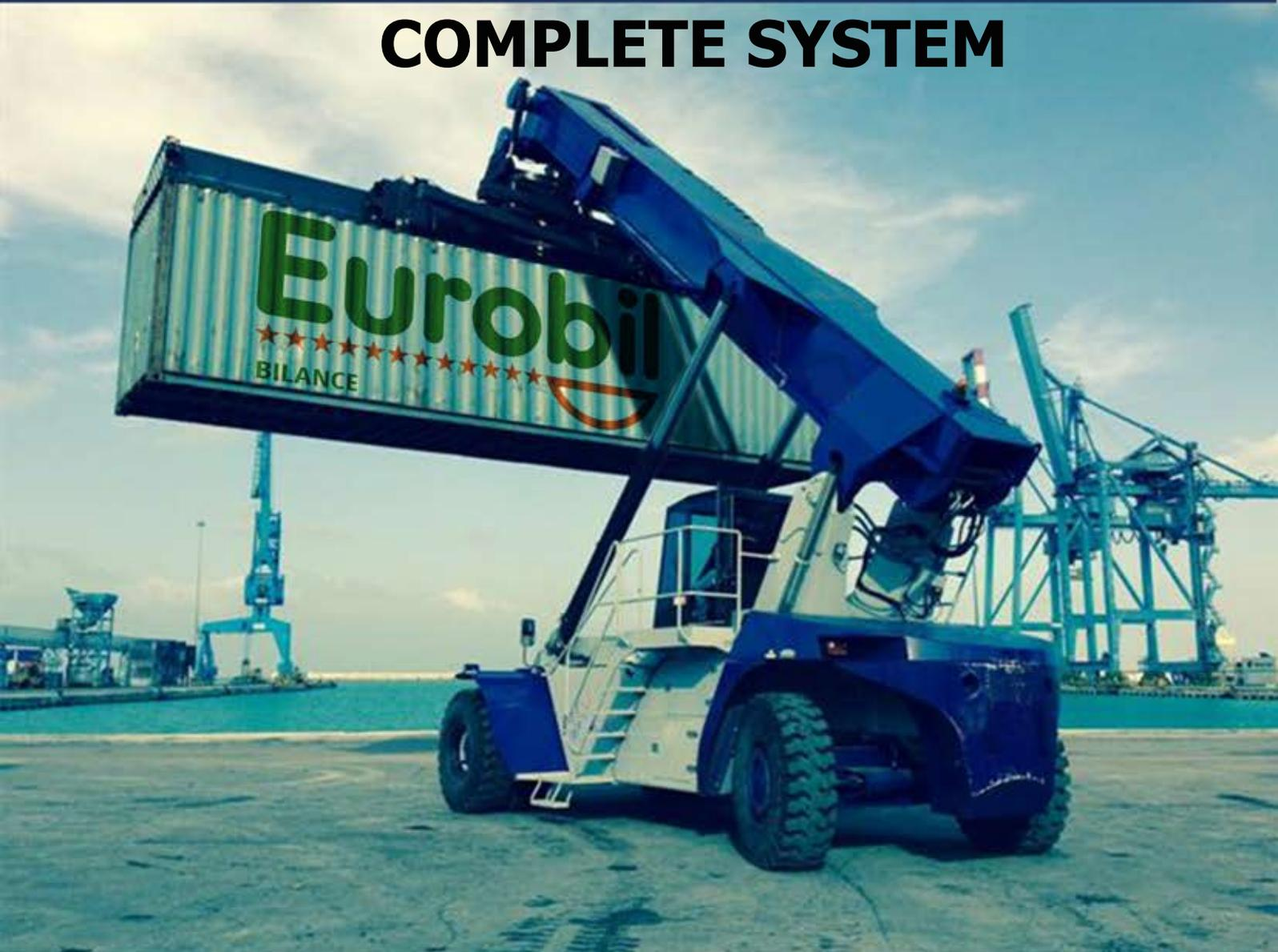
Possibility of connecting 4 or 8 weighing twistlock for individual spreader or twinlift
